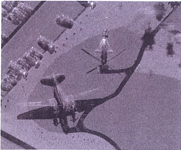
Figure 14-44: Example of how a shadow can reveal the shape of the object creating the shadow. The radar illumination direction is from the top of the image. [Image courtesy of Sandia National Laboratories.]
