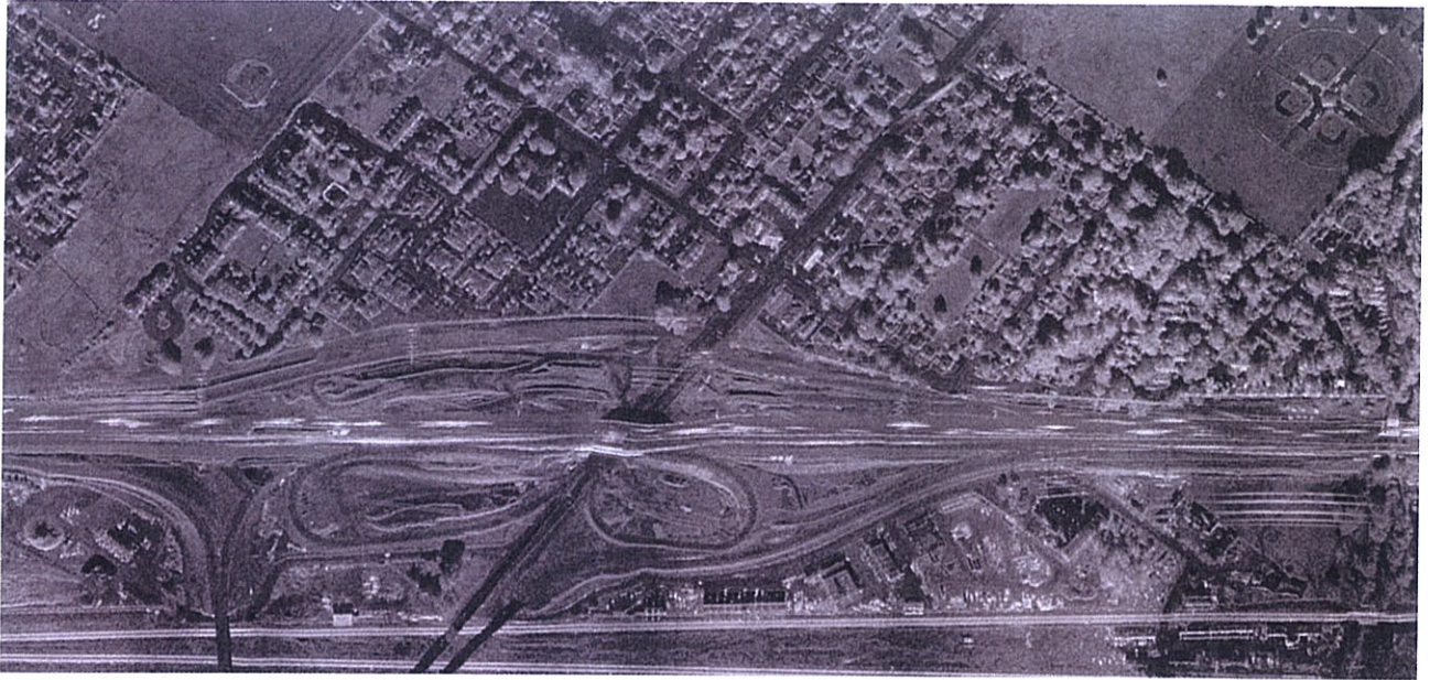
Figure 14-43: Multilook SAR image with image distortions due to digital elevation model (DEM) errors. The bridge at the center is distorted since it is not included in the DEM. Streaks along the freeway are due to moving vehicles. Parallel lines at the bottom are railroad tracks.
